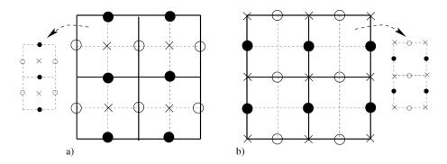
Fig. 2. Fine and coarse grid cells and staggered grid unknowns, o:  $u_H$  point,  $\bullet$ :  $v_H$  point,  $\times$ :  $p_H$  point; (a) for Stokes, (b) for poroelasticity.
